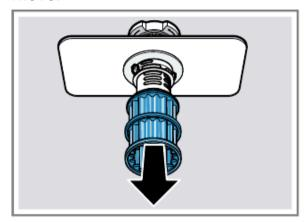
4. Press the locking catches ① together and lift the coarse filter out
